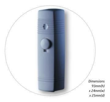
VIBRO is an intelligent, microprocessor-controlled shock sensor suitable for a variety of internal applications. The unit is easy to install, featuring a unique 'Learn Mode' function, which automatically sets the sensitivity by 'learning' the level and number of impacts required to generate an alarm. Multiple impacts can be overridden using the 'Gross Attack' feature, which enables VIBRO to create an alarm from a single impact.
