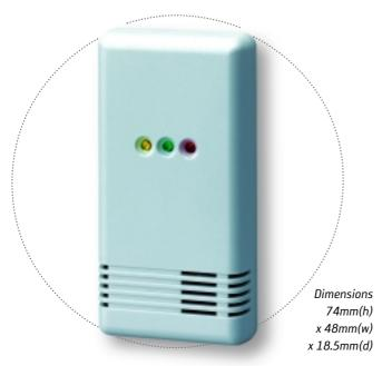
The GX-252T is a microprocessor-based glassbreak detector utilising dual frequency analysis to detect the common sounds of shattering glass and acoustical shock when a window is broken. The sensor only activates when specific frequency patterns continue for a fixed time period, making it highly immune to false alarms.
