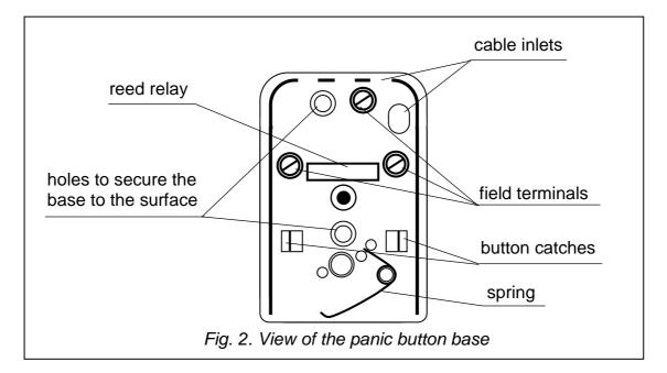
**CAUTION!** Be particularly careful during installation so as not to damage the glass enclosure of reed relay or the magnet situated on the button.
