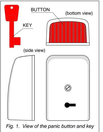
casing until it is released with the key. Where a few buttons are connected to one zone of the alarm control panel, this function makes it possible to identify the button which triggered the alarm.
