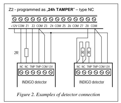
Figure 2 shows typical examples of connecting the detectors in EOL (parameter) configuration and 2EOL (two-parameter) configuration. Resistors should be mounted inside the detector housing.
